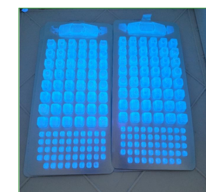
Figure 4: Quanti-Tray®/2000 System with Strong Fluorescence: High Enterococcus Levels in High Septic System Ditch [HSD] water sample.
