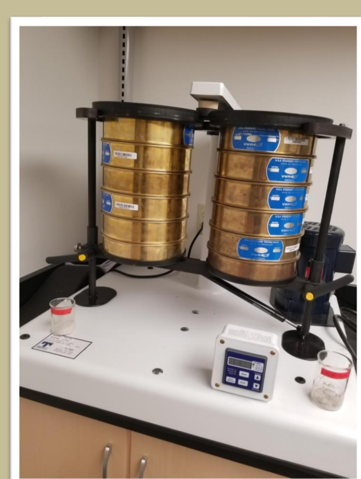
The dry sand samples were in the sieve shaker for 15 minutes.
