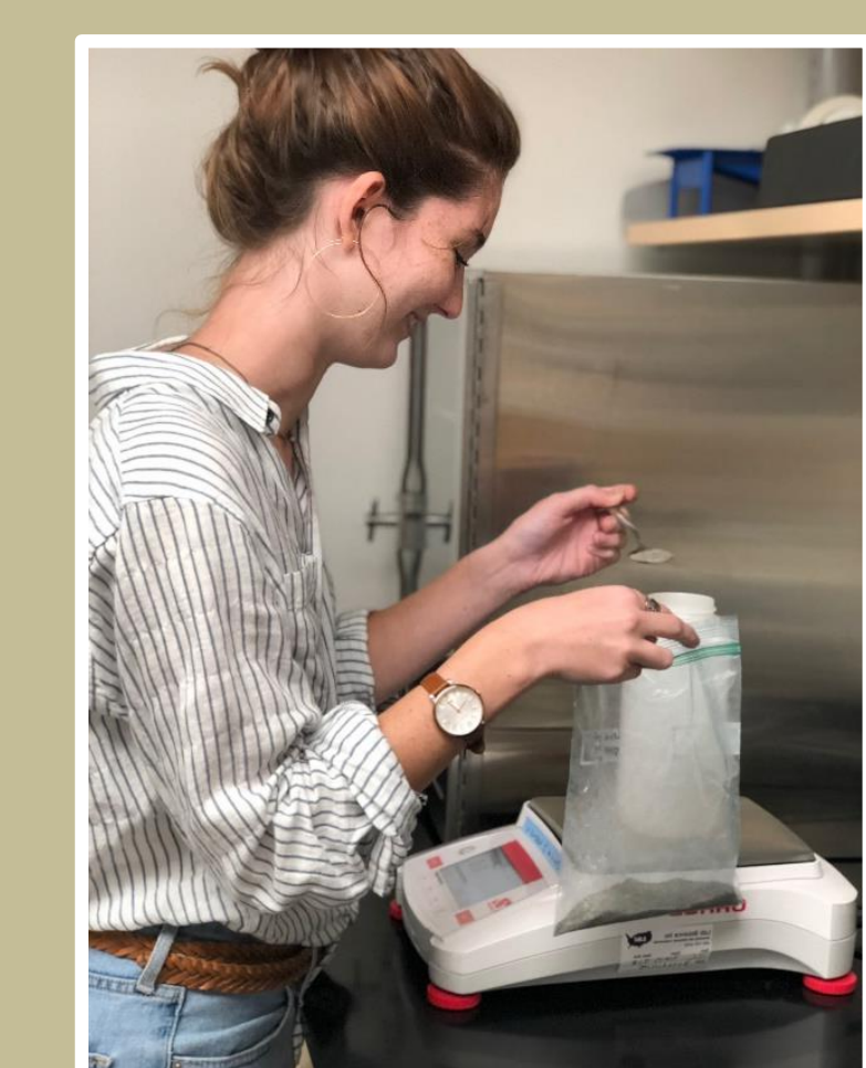
30 g of sediment was measured into a Nalgene bottle.
