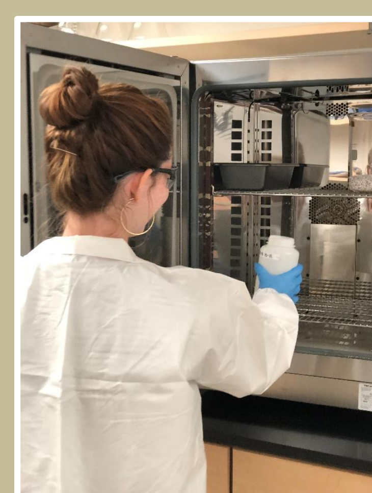
The sediment mixed with concentrated hydrogen peroxide was placed in the oven overnight to dry.
