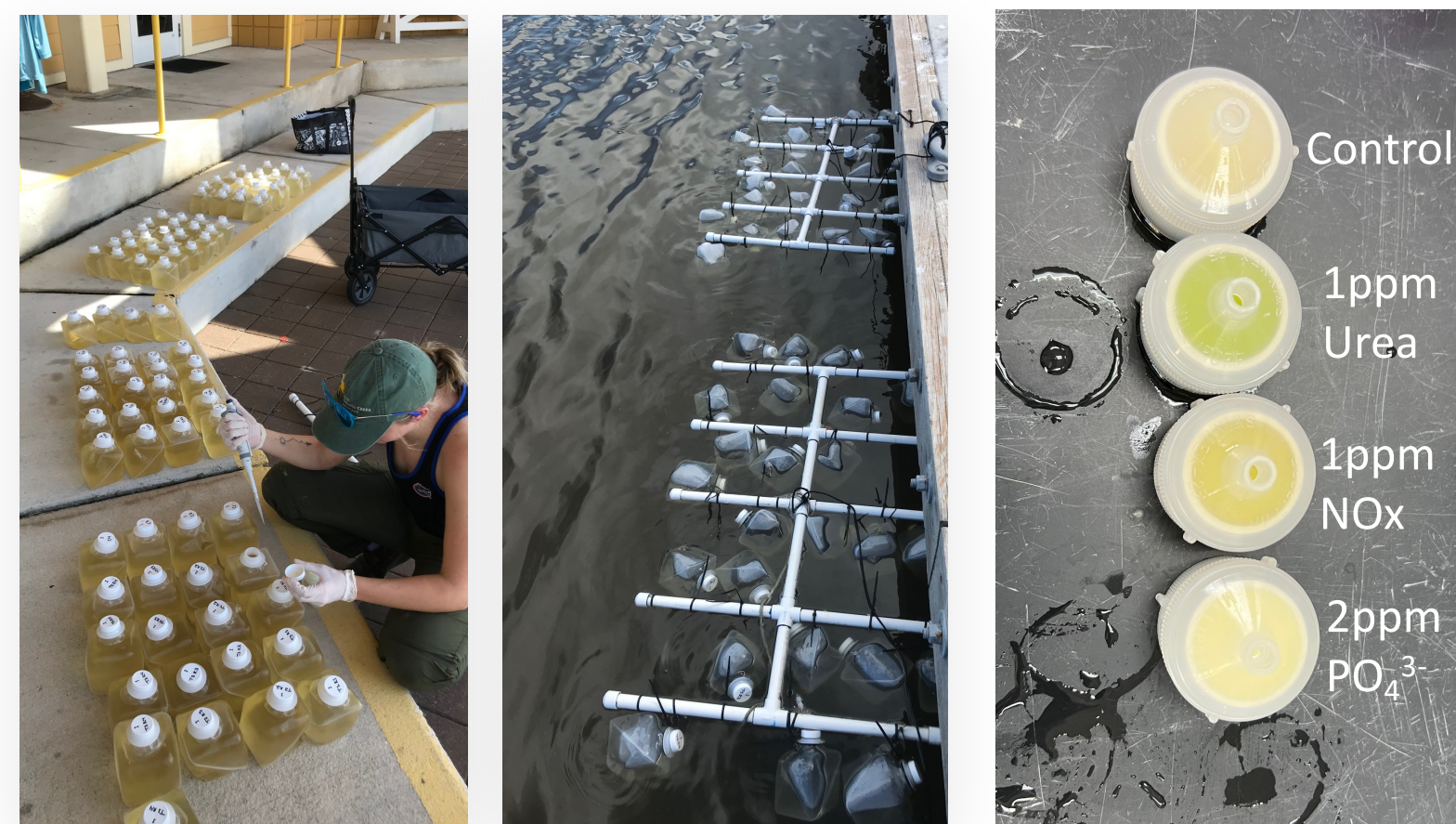
Figure 3. Cubitainers filled from each site, dosed with different nutrient treatments and then deployed together to incubate for 2.5 days.
