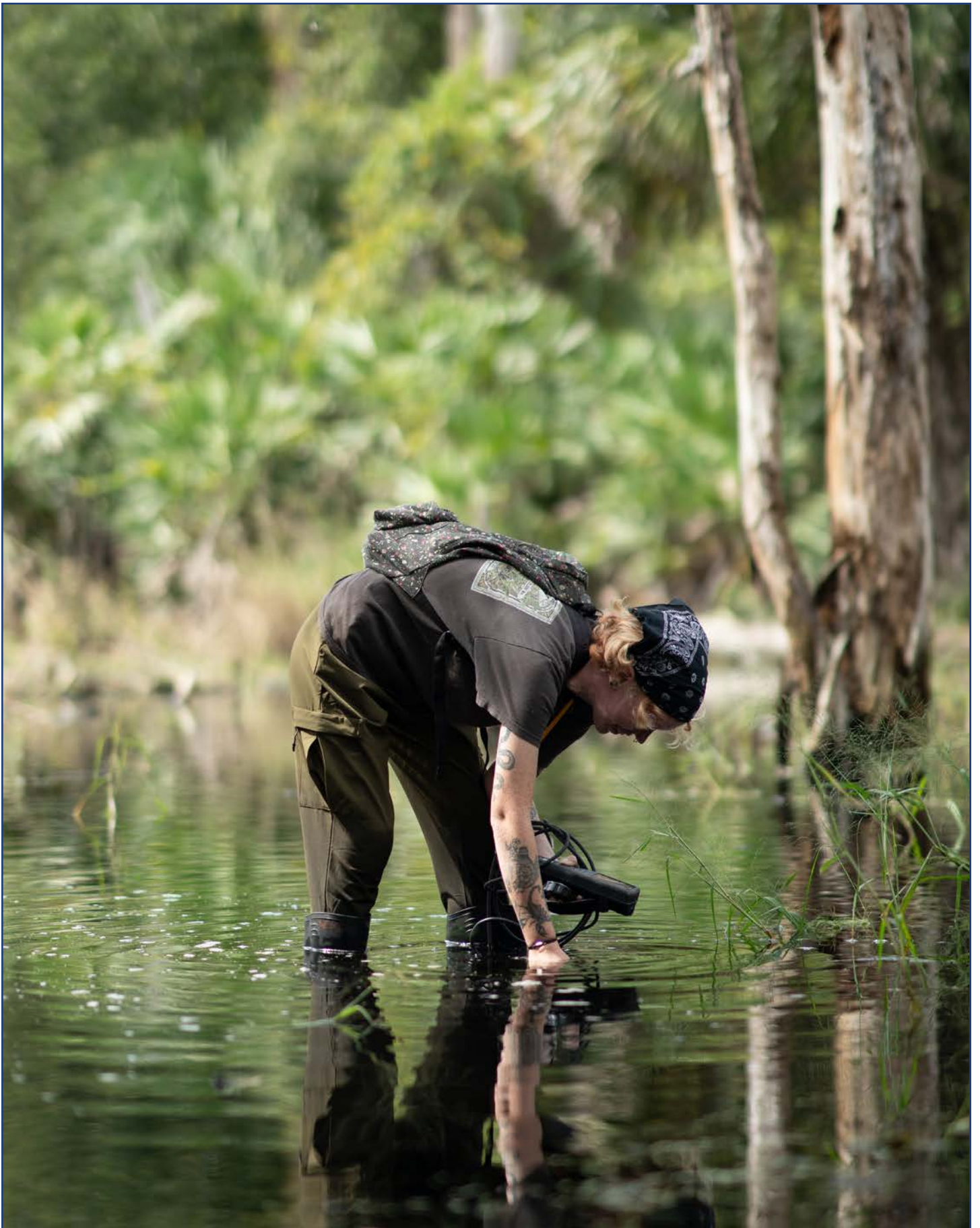
Elizabeth Terwillinger collects surface water quality data using a YSI ProDSS instrument. Photo by Emily Hill.
