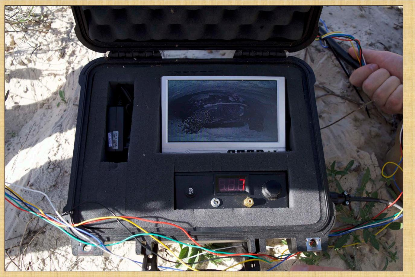
We find that the current robot is only effective in larger burrows; design changes will make it more accessible to smaller burrows in the future. Our "BurrowBot" makes capturing footage more efficient, and maintains the camera's orientation effectively, meaning less post-production of photos is needed.
