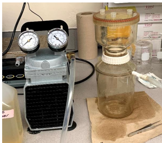
Figure 3- Vacuum Filtration Apparatus
