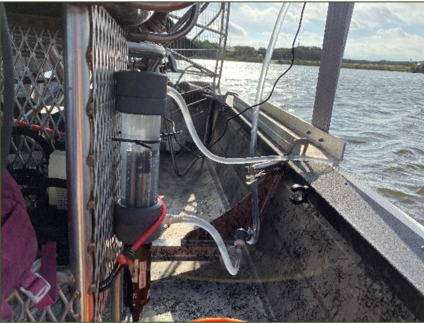
Flowcell system with multiple water quality sensors
