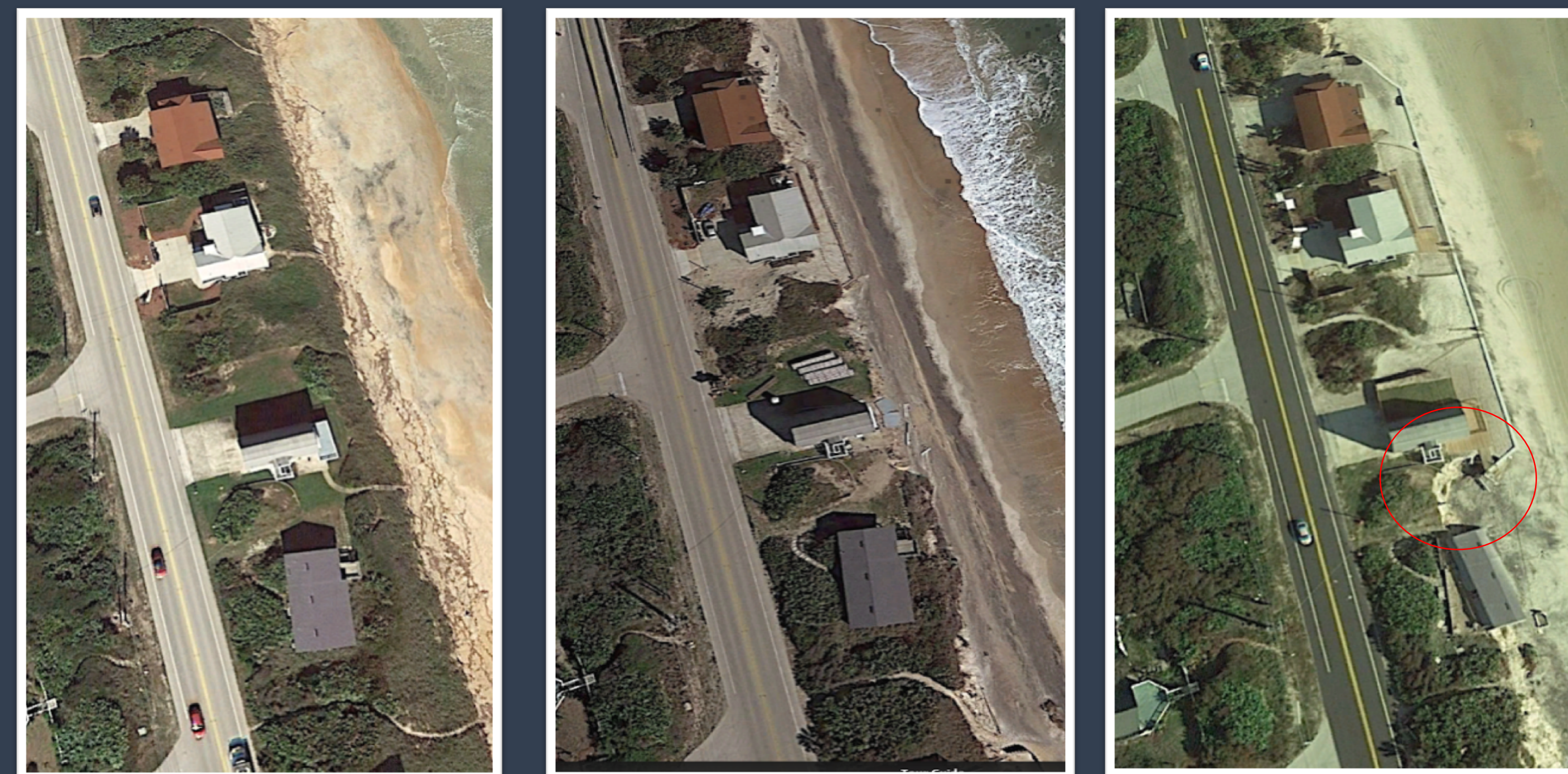
Image 1: For future studies we would like to look at post Hurricane Irma satellite images to help further conclude our hypothesis. Shown above are satellite images, to the left shown by the red circle is the progress of erosion after sever weather events directly adjacent to a hardened structure.
