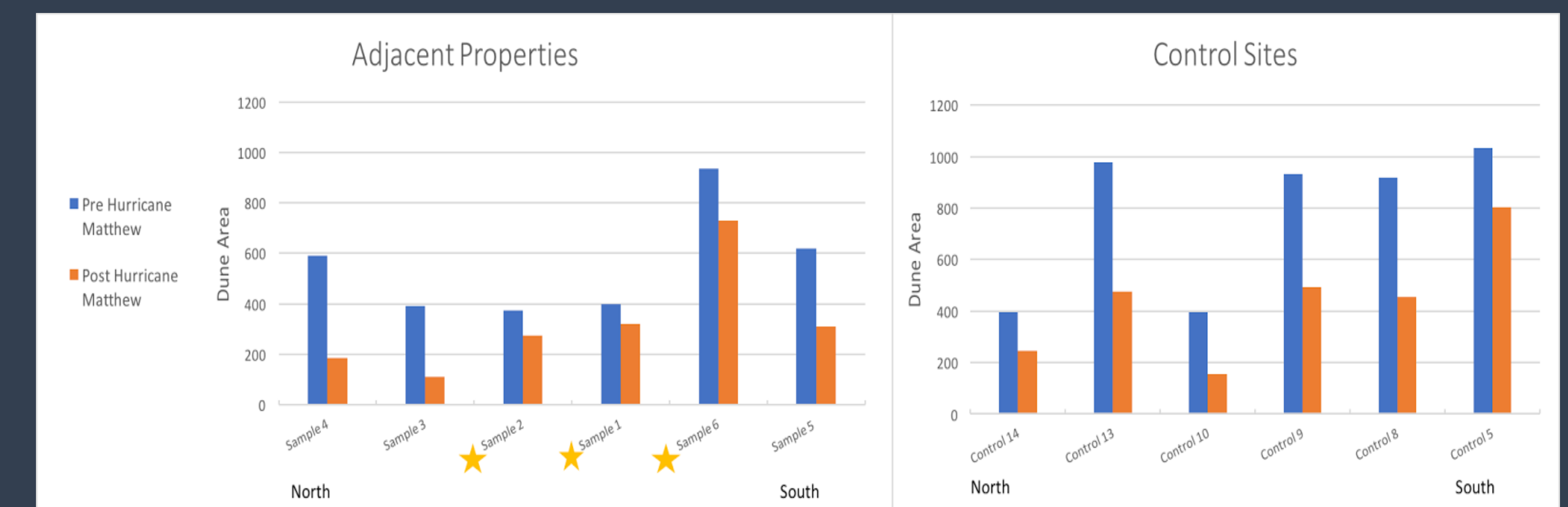
Graph 3: Geospatial analysis between pre Hurricane Matthew (2014) and post Hurricane Matthew (2017) satellite images, North of each individual hardened structure properties (left) and control sites (right). Yellow stars represent hardened structures constructed of rocks rather than a wall. P-value of hardened structure properties is 0.049 and P-value of control sites is 0.01 mean we can accept the hypothesis that there was erosion following Hurricane Matthew.
